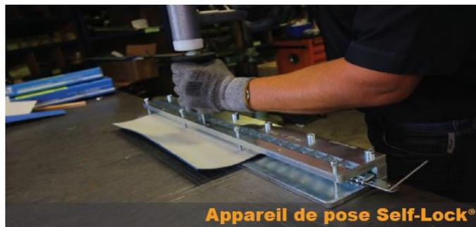
**Appareil de pose Self-Lock®**
